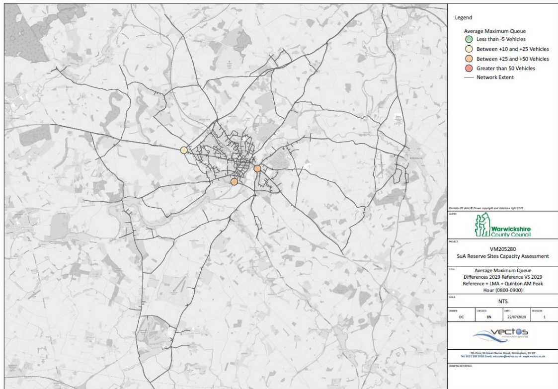
Figure 4 Queue Length Analysis – 2029 Reference Case vs 300 LMA + 250 South of Stratford + 200 Quinton Area (AM Peak Hour)
