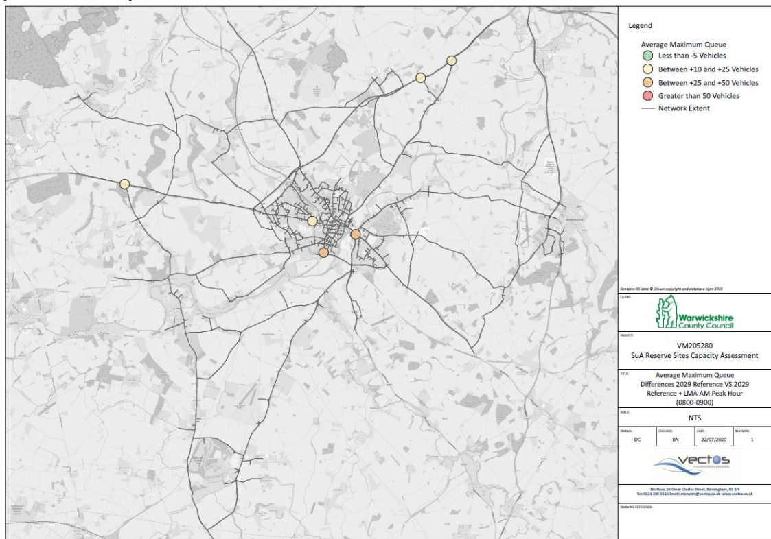
Figure 2 Queue Length Analysis – 2029 Reference Case vs 2029 Reference Case + LMA 750 (AM Peak Hour)
