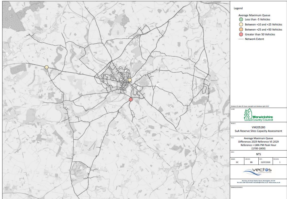
Figure 3 Queue Length Analysis – 2029 Reference Case vs 2029 Reference Case + LMA 750 (PM Peak Hour)
